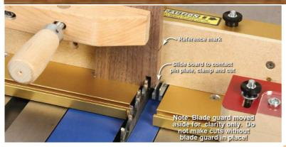
Once set up make a sample cut with your saw blade or Router bit, Metric or Imperial, as your iBOX automatically adjusts to both dimensions.
