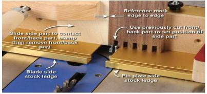
Unclamp board and set previous cut over pin plates. Re-elamp and cut again
